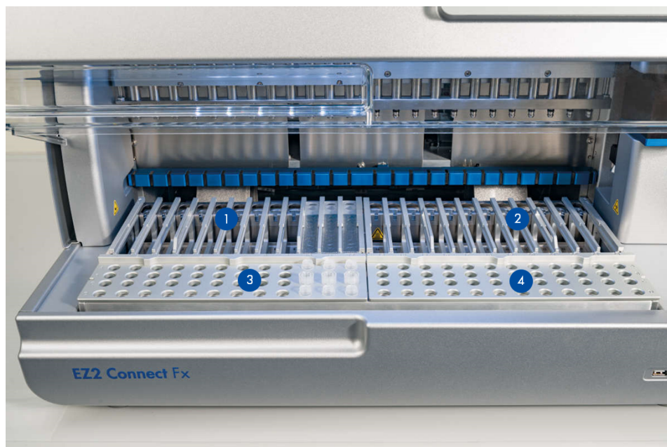
Figure 2. EZ2 Connect worktable. [1] EZ2 Connect Cartridge Rack, left. [2] EZ2 Connect Cartridge Rack, right. [3] EZ2 Connect Tip Rack, left. [4] EZ2 Connect Tip Rack, right.
