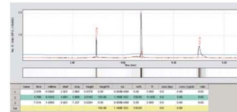
Figure 7. Electropherogram showing specific PCR product. Genomic DNA purified from dog teeth was used as template in a real-time PCR assay for \beta -actin. The final PCR product was analyzed on the QIAxcel using a QIAxcel DNA High Resolution Gel Cartridge and AM 0112 Alignment Marker 15 bp/5 kb. Detection was carried out using the OM500 method (5 kV per 500 seconds separation time). The central peak indicates the specific PCR product. The left- and right-hand peaks indicate the alignment markers.
